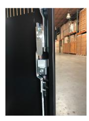
Remove the screw (1) from the bottom of the lock assembly that holds the u-shaped retaining bracket.
