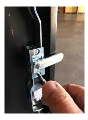
Once the screws have been remove lift off the front half of the lock assembly and set it aside.
