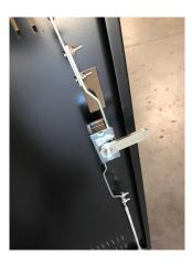
Remove the two (2) screws and nuts holding the rods to the lock assembly and transfer to the new lock assembly.
